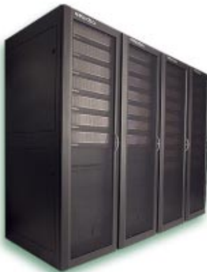
Figure 2. Capable of scaling to hundreds of terabytes of data, the Netezza Performance Server system also scales in processing performance to power critical BI applications. Shown is the four-rack NPS 8450 system.
