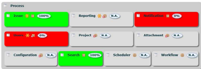
Fig 6: Identification of untested changes. Analysis of changes is crossed with test coverage. In this example, changes in the Notifications or Users subsets have not been tested.
