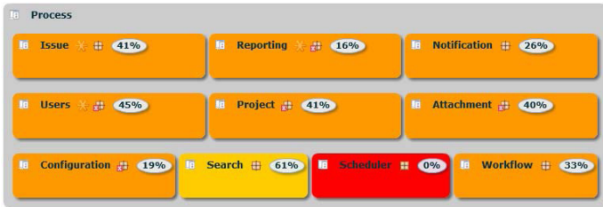
Fig 5: Identification of untested or poorly tested areas. Here the general coverage of functional subsets by testing. In this example the Scheduler subset has not been tested.
