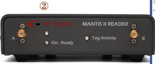
▲ Warner Robins Air Logistics Center deployed an RFID system for tracking gyroscopes that go into aircraft. The platform was built by RF Code and includes hundreds of active RFID tags (I), which communicate data to I9 Mantis readers throughout the facility (2). From there, information goes through RF Code's Tavis Data Management software (3), which integrates with the DOD's Automated Materiel Tracking System.
